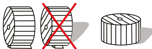
Do not lay cable drums on flat on their sides, use proper stops to prevent drums rolling.
